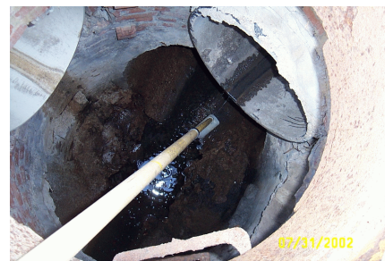
Figure 15. Collecting a sample using telescoping sampling pole.
